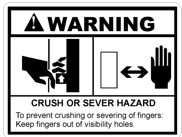
PART #41112 WARNING! CRUSH OR SEVER HAZARD
